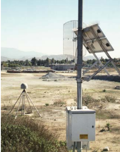
Figure 6. Remote CGPS site with antenna aimed toward backbone site (left) and backbone antenna on roof of building with LAN connection aimed at CGPS site (right).
