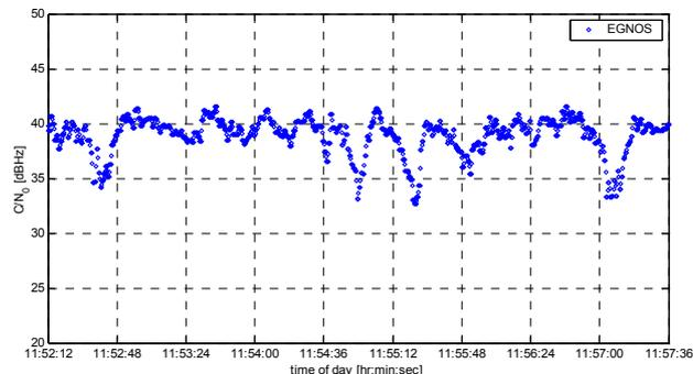
**Figure 7: carrier to noise ratio of the EGNOS satellite**
