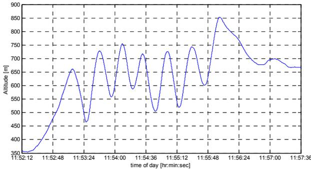
**Figure 6: height variations during the parabolic manoeuvring**
