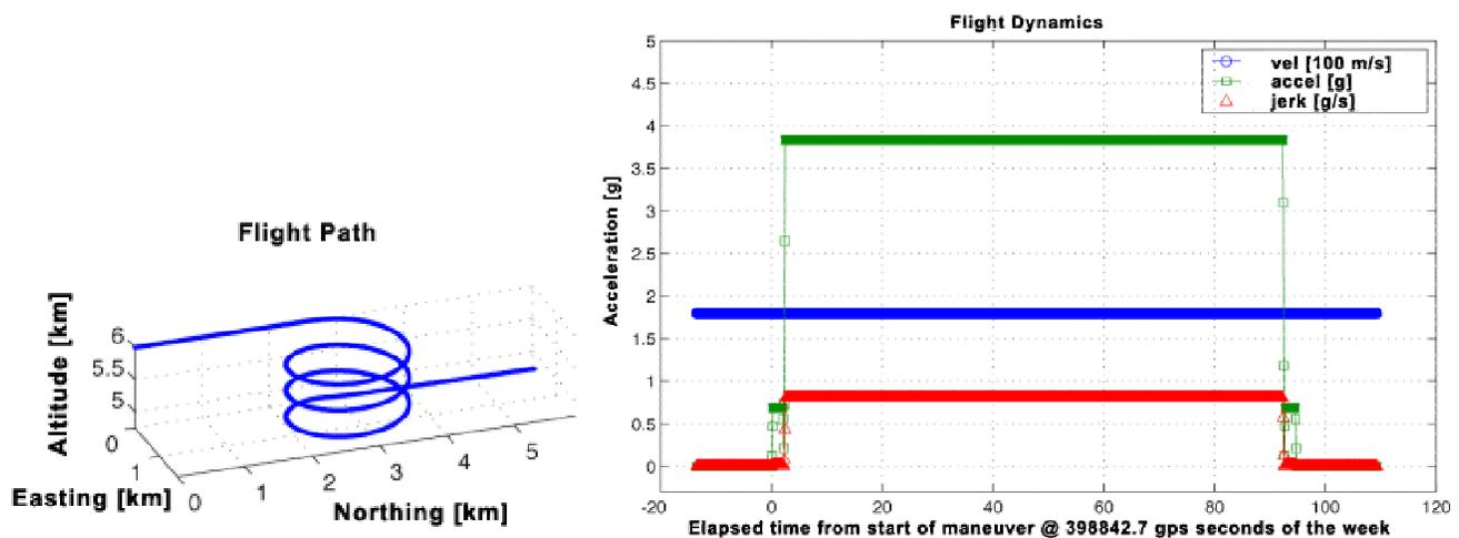
**Figure 3.** Rover flight path and dynamics of the “Post/Hole” maneuver with up to 4g’s of acceleration. The velocity is kept constant at 100m/s, while the acceleration and jerks were varied.
