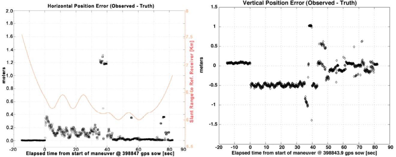
Figure 9. Near position errors for “9g Turns” maneuver in graceful degradation mode
