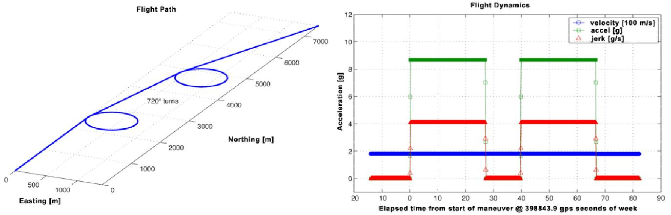
**Figure 4.** Rover flight path and dynamics of the “9g Turns” maneuver with up to 9g’s of acceleration. The velocity is kept constant at 100m/s, while the acceleration and jerks were varied.
