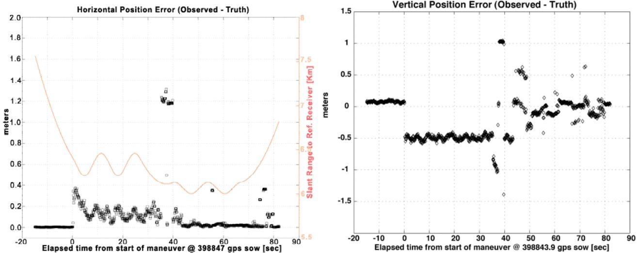
Figure 9. Near position errors for “9g Turns” maneuver in graceful degradation mode
