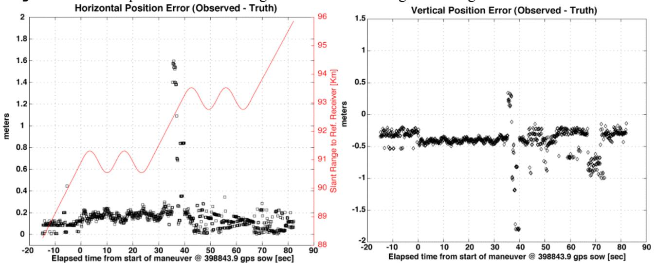
Figure 10. Far Position errors for “9g Turns” maneuver in graceful degradation mode
