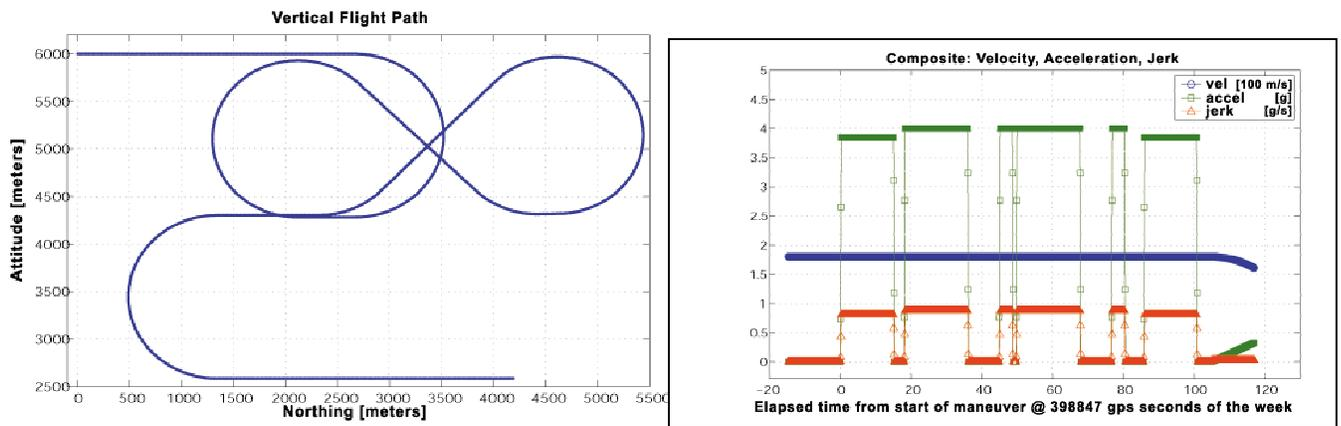
**Figure 2.** Rover flight path and dynamics of the “Split S-Cuban 8-Split S” maneuver with up to 4g’s of acceleration. The velocity was kept constant at 100m/s, while the acceleration and jerks were varied.
