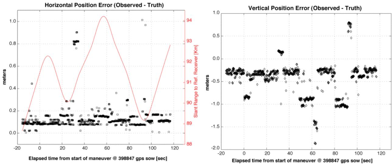
Figure 6. Far position errors for “Split S-Cuban 8-Split S” maneuver
