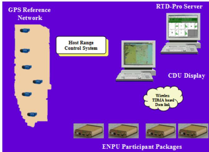
with the wireless data-link to both transmit the GPS observables produced by the reference network to the participant packages for their use in the positioning process, as well as a mapping solution showing the computed location of the participant packages.
