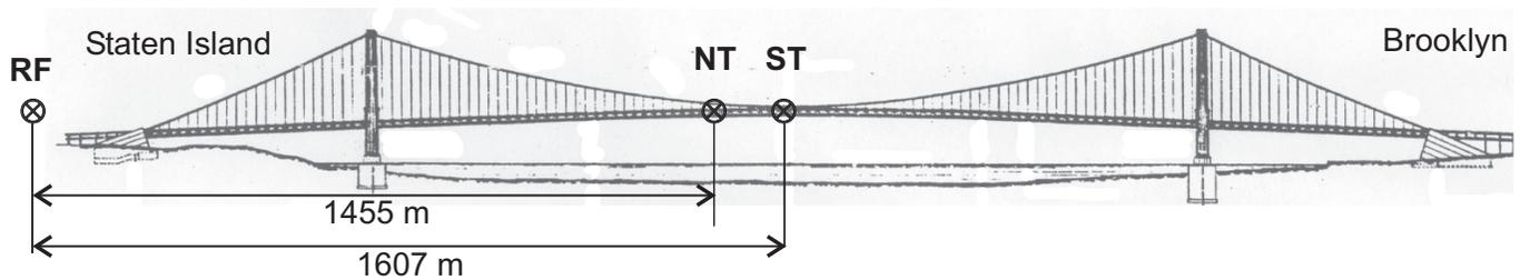
▲ **Figure 1.** Location of GPS antennas on the bridge. GPS antennas were installed at stations NT (northern truss), ST (southern truss), and RF (Staten Island). Observations at NT and ST were processed with respect to RF.
