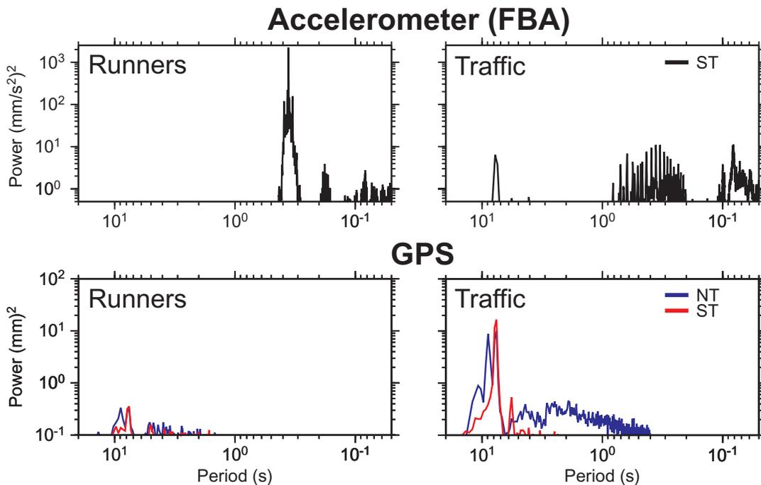
▲ **Figure 5.** Power spectra of vertical oscillations of the deck from observations with force-balance accelerometers (FBA) and GPS.
