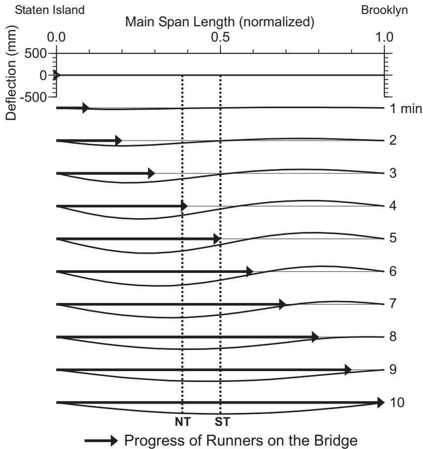
▲ **Figure 4.** Evolution of predicted vertical deflection of the deck during the period of loading by runners at various points on the bridge. For each vertical cross-section, the time elapsed since the beginning of loading is labeled on the right. Prediction is based on the second-order deflection theory. The best fit with observed deflections is achieved using the uniform live load 4.4 kN/m ( $p = 0.3$  kips/ft).
