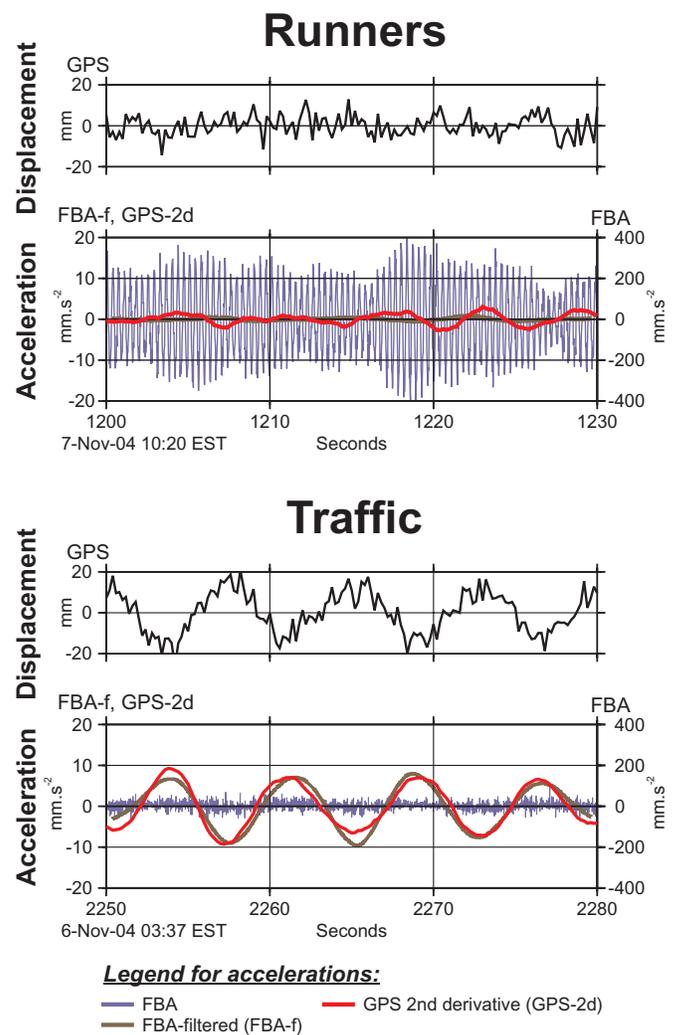
▲ **Figure 6.** Oscillations associated with the natural frequencies of the bridge, excited by runners and by traffic. Displacements are shown as observed with GPS. Accelerations are shown in three manners: 1) observed with FBA; 2) FBA low-pass filtered with a corner period of about 1 s; and 3) the second derivative of GPS displacements.
