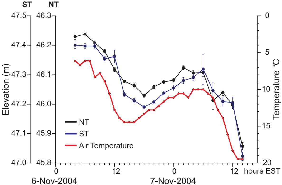
▲ **Figure 8.** Variations of one-hour averaged elevations of NT and ST, and variations in one-hour averaged air temperature. Hourly GPS solutions were performed by GAMIT (King and Bock 2005) with respect to station RF (figure 1).
