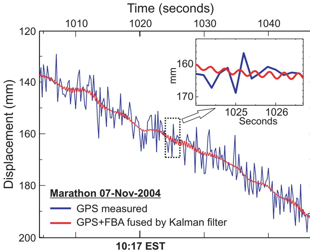
▲ **Figure 7.** GPS measured displacements, and GPS + FBA displacements fused by Kalman filter.
