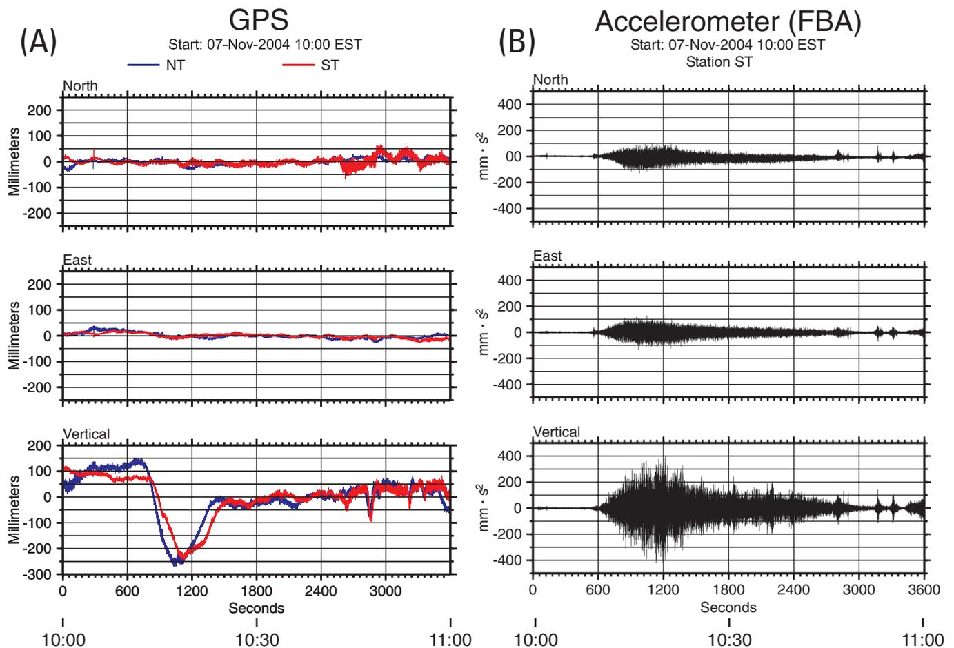
▲ **Figure 3.** A: Three components of deflection of the bridge deck under load of runners from GPS solution. Corrected for multipath. B: Three components of vibrations of the deck excited by runners, measured by the force-balance accelerometer (FBA).
